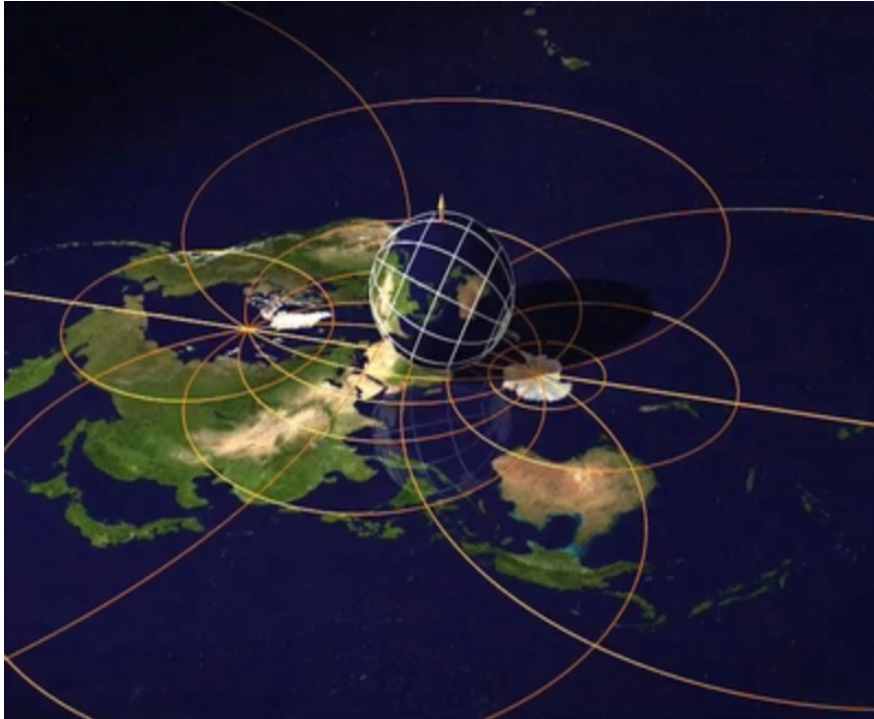
Distortion of different areas of the earth under the stereographic projection
