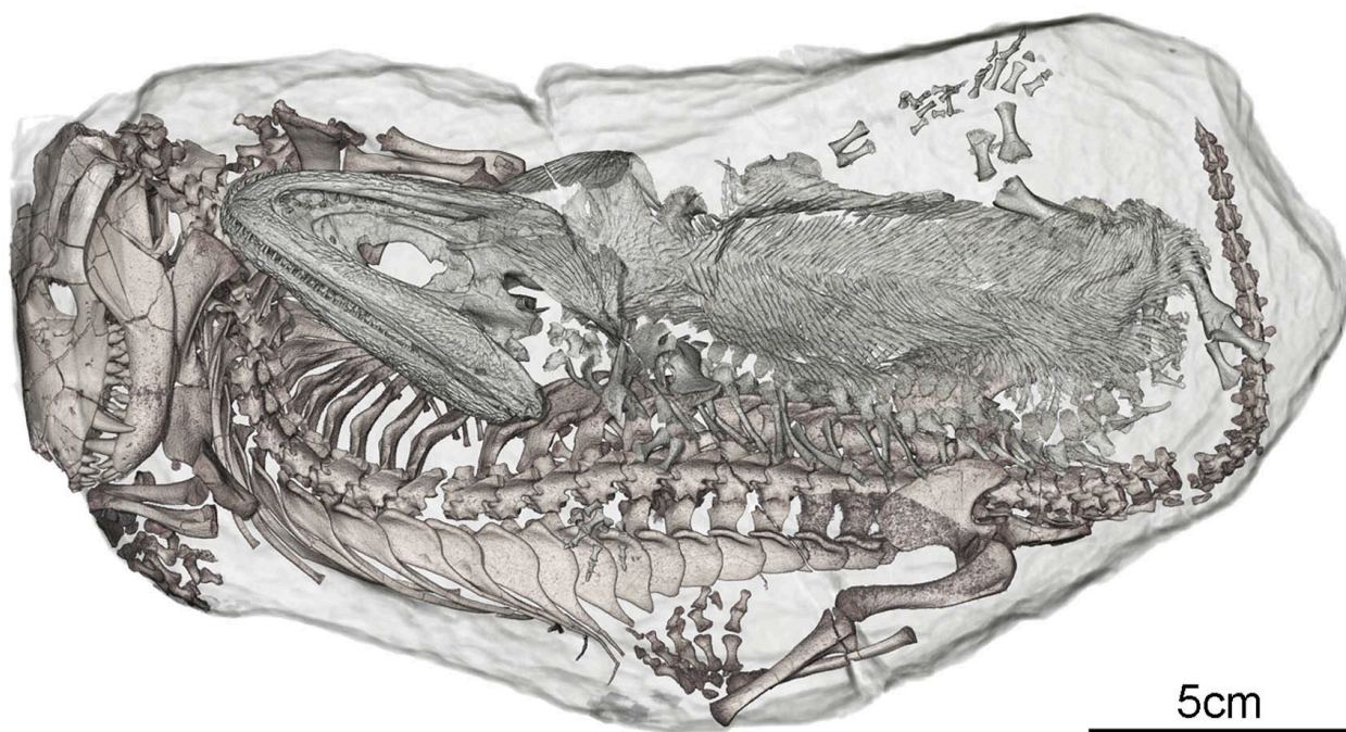
Figure 4: Synchrotron image of a burrow containing two fossil skeletons (Fernandez et al. 2013, 2).
