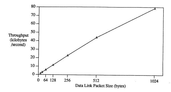
Figure 6 - Data Link Throughput vs. Data Link Packet Size
