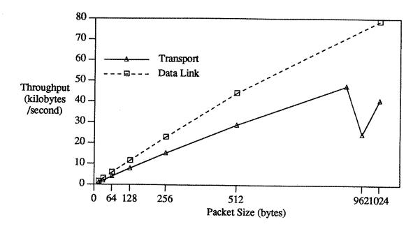
Figure 11 - Transport and Data Link Throughput vs. TSDU and Data Link Packet Sizes
