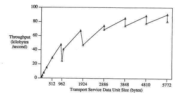
Figure 7 - Transport Throughput vs. Transport Service Data Unit Size
