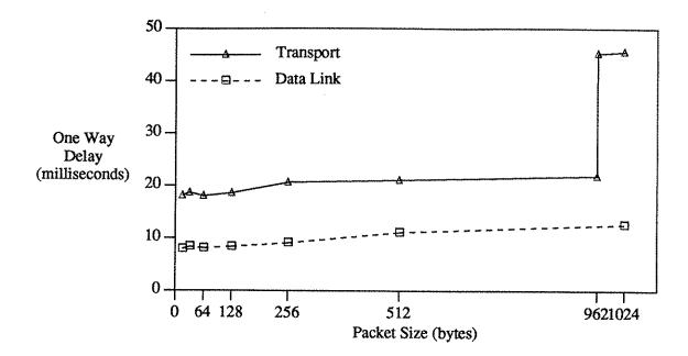
Figure 10 - One Way Transport and Data Link Delay vs. TSDU and Data Link Packet Sizes
