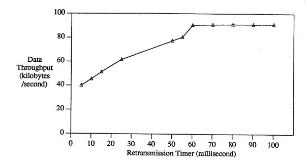
Figure 8 - Transport Throughput vs. Setting of the Retransmission Timer
