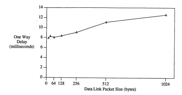
Figure 4 - One Way Data Link Delay vs. Data Link Packet Size
