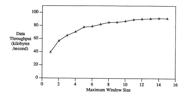
Figure 9 - Transport Throughput vs. Maximum Window Size
