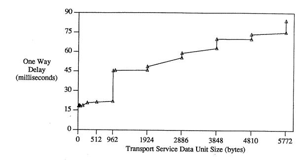
Figure 5 - One Way Transport Delay vs. Transport Service Data Unit Sizes
