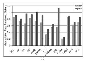
Figure 15: Relative IPC and misprediction rates for the 12 SPEC2000 integer benchmarks for the hashed, path-based and gshare predictors. Note that the gshare predictor is 16kb while the two perceptron predictors only have a 10kb storage budget.
