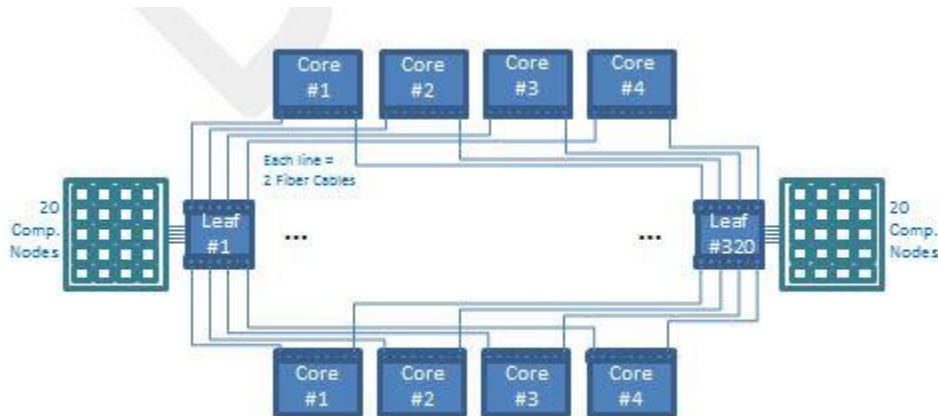
Figure 3: Stampede's Interconnection Structure (Source: Texas Advanced Computing Center)
