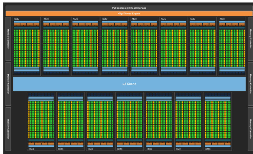
Figure 2: Block diagram of a NVIDIA Kepler GPU having 15 symmetric multiprocessors (Source: NVIDIA Website)
