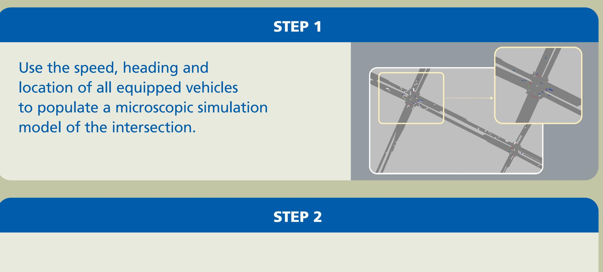
Simulate vehicle positions 15 seconds into the future, including the necessary yellow and red time for a signal change.
