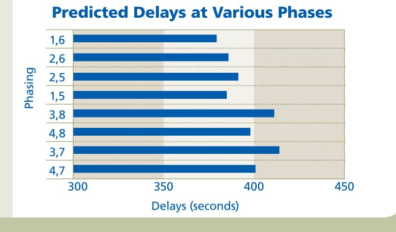
Select the phase with the lowest predicted cumulative delay as the next phase. Each phase has a maximum red time of 120 seconds, and disruptive queues trigger an immediate green.
