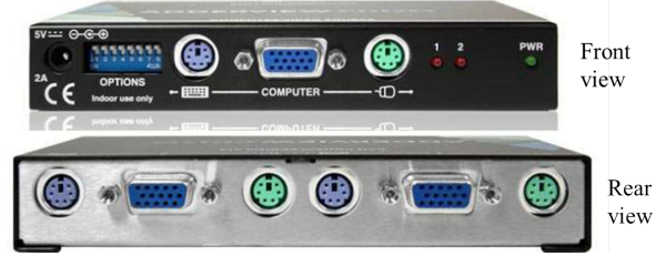
(d) Front and rear views of a reverse-KVM switch [12]
