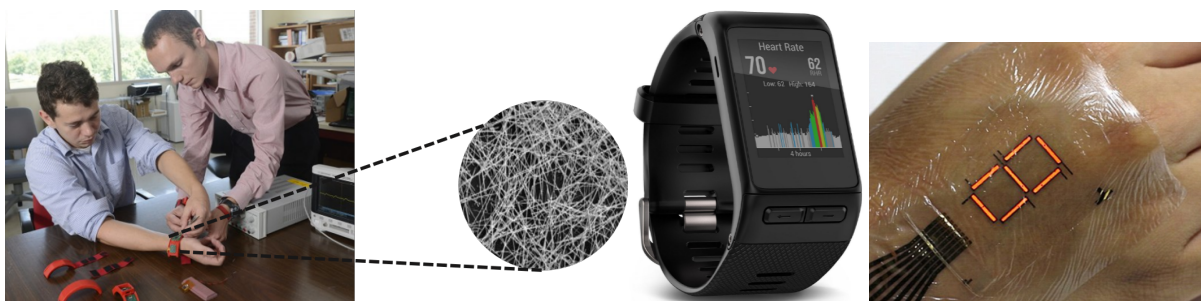
Figure 2. EKG and EMG data collection prototype with images of the nanosilver wires that conduct electrical signals from the skin to the device mounted on a wristband.
