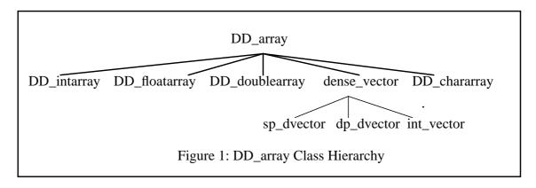
One of the most important services that can be provided by a library for use in a parallel/distributed environment is the ability to decompose the data to be sent to the various processors. The class DD\_array provides functions that allow the user to decompose the matrix into one of five forms: by row, by column, cyclically by row, cyclically by column, or by block.
