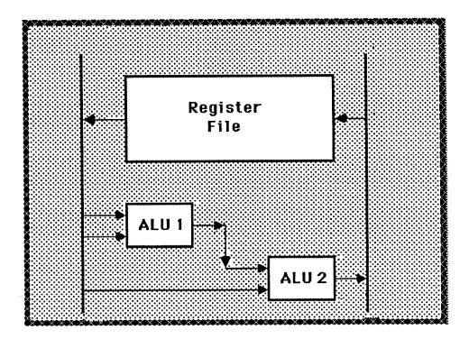
The pipelined structure of the WM execution units induces the data dependency rule:
