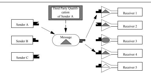
FIGURE 3. The general decoupled communication paradigm of Selective Notification.
