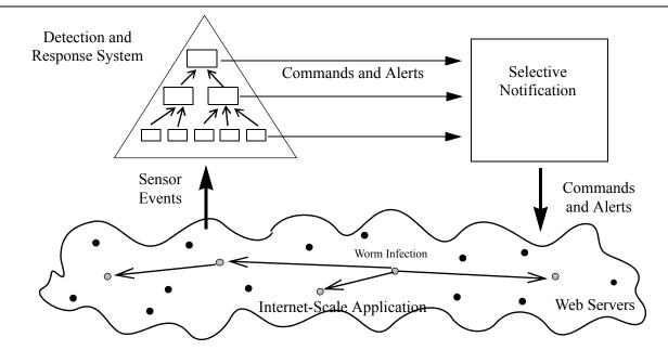
FIGURE 1. Survivability of Internet-scale distributed systems with survivability architecture.
