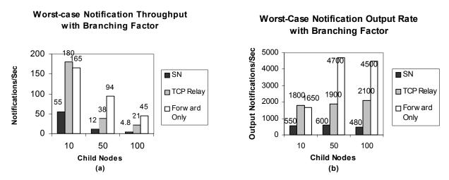
FIGURE 7. (a) Worst-case event throughput with forwarding-set size; (b) Worst case event forwarding rate with forwarding-set size.
