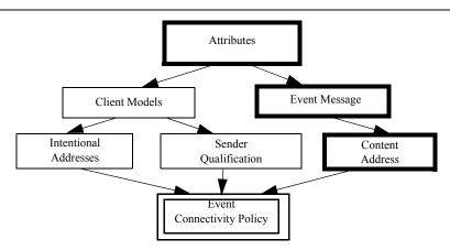
FIGURE 4. The composition of Selective Notification and Siena elements.
