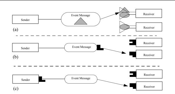
FIGURE 2. Decoupled event communications in (a) content-driven publish/subscribe; (b) intentionally addressed messaging; and (c) sender qualification.
