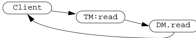
(b) Call graph illustrating communication for TM:read. Arcs represent message traffic.
