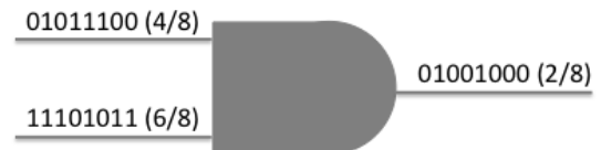
Figure 11: Approximate multiplication of two stochastic input streams [1]. This example illustrates inexact computation of 4/8 \times 6/8 .
