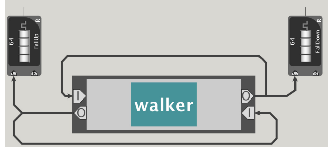
Figure 8: A linear Markov chain walker bounded by counters. This construction can represent discrete values with arbitrary precision without a linear increase in states.
