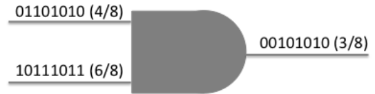
Figure 10: Approximate multiplication of two stochastic input streams [1]. This example illustrates exact computation of 4/8 \times 6/8 .
