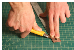
Snapping off a blade segment.
