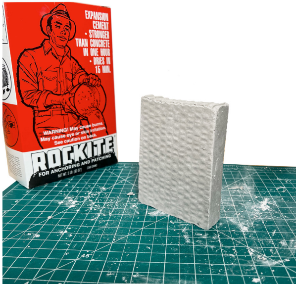
Completed cast (note rippled face due to moisture warping face of corrugated cardboard mold).
