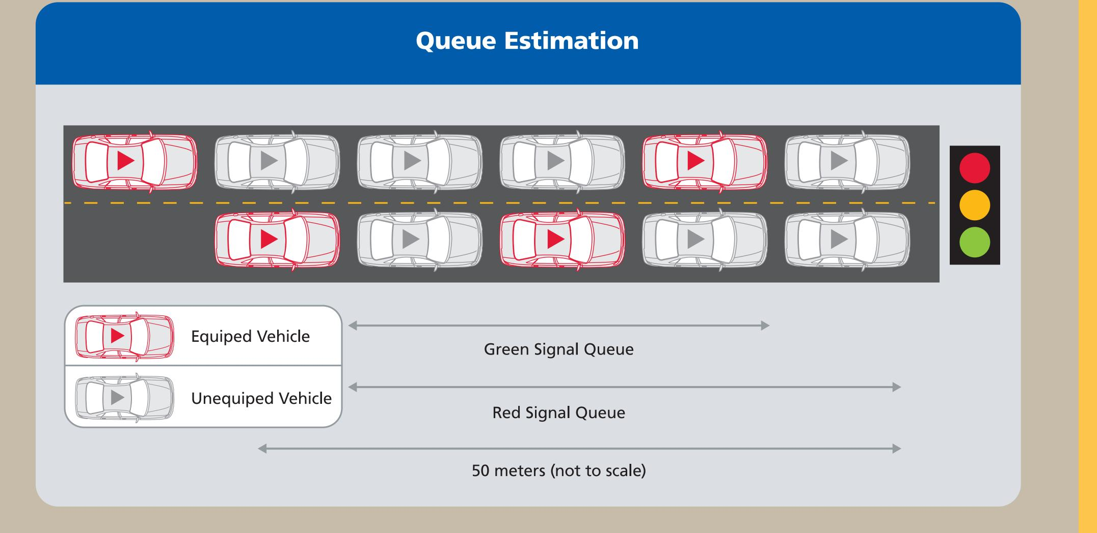
**Step 2:** Estimate Vehicle Speed and Location. The gaps in the queue are assigned simulated unequipped vehicles (called "inserted vehicles"), with speeds of zero, lengths of 4.75 meters, and gaps of 2.5 meters.
